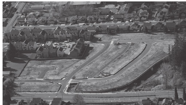
New subdivision of homes - Roads, utilities, and other infrastructures built prior to the construction of the homes.
