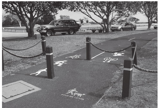
There may also be places where physical barriers are necessary to slow bicycle traffic down.
