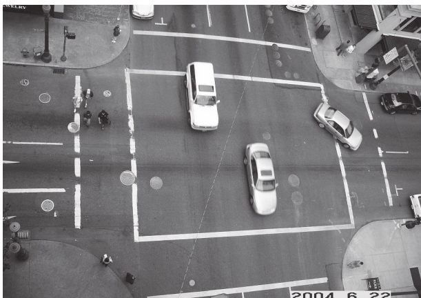
Numerous manhole and valve covers - an indication of all the hidden utilities beneath this intersection
